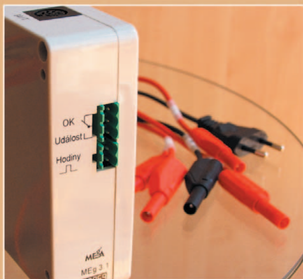
MEg 31 - portable version for MV networks
