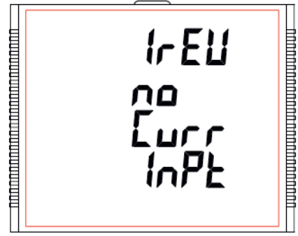
This screen shows that the meter has no current input.
