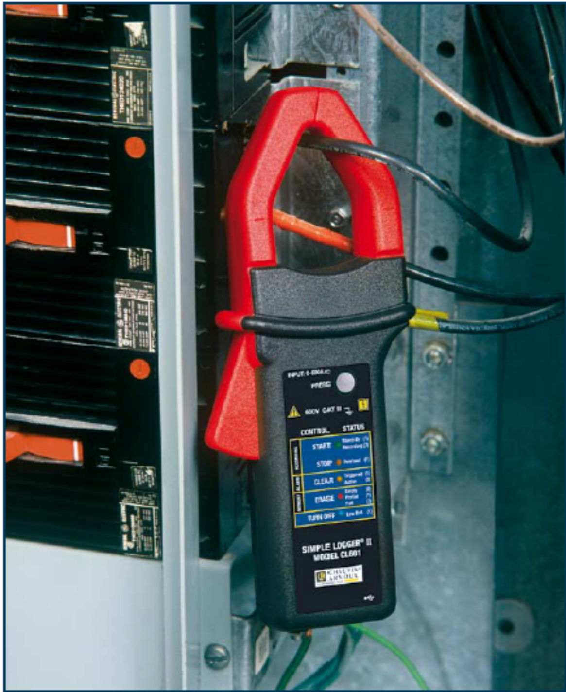
Easily log current in power panels.
