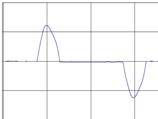
Figure 5. Current for an electronic load.
