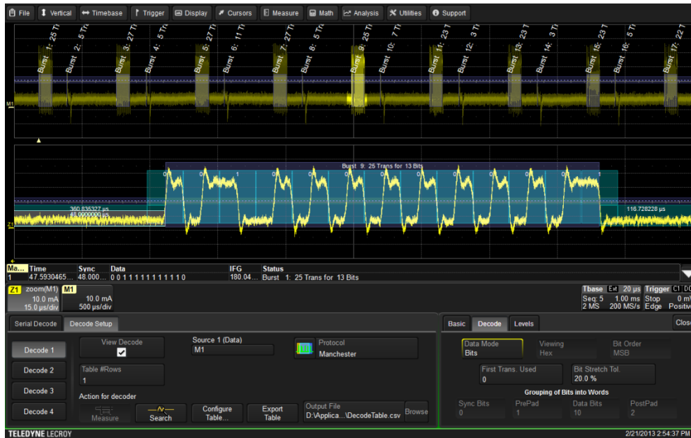
Figure 5: Verifying correct bit-level decode with a zoomed view
