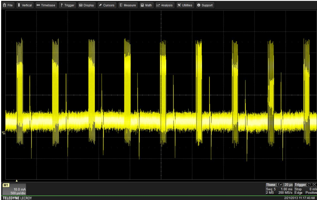
Figure 1: A PSI5 signal with 13-bit data frame
